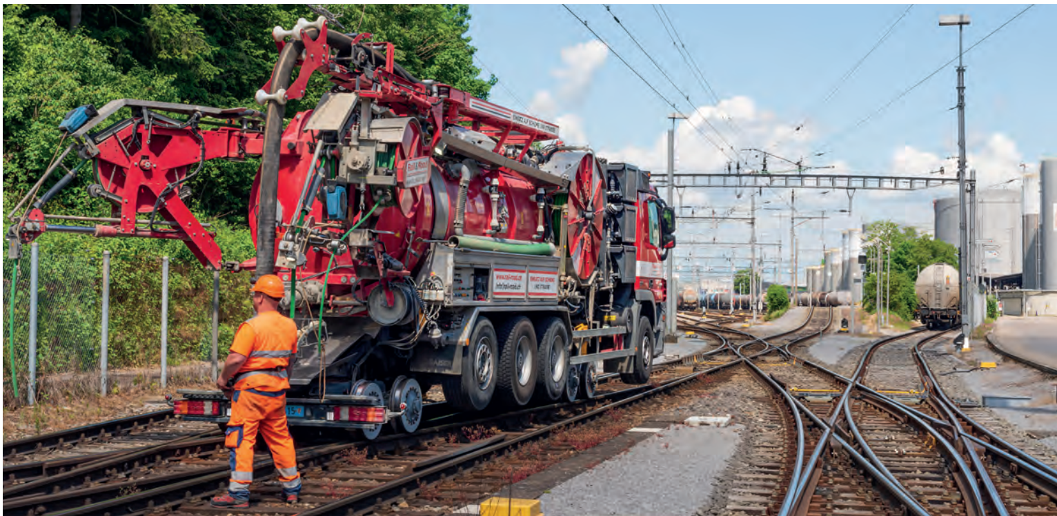
Separation into water and solid materials through the addition of flocculants and multiple filtration.
